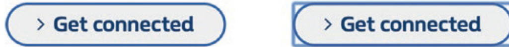
Figure 4-1. A picture of a button and then that same button with keyboard focus style applied
